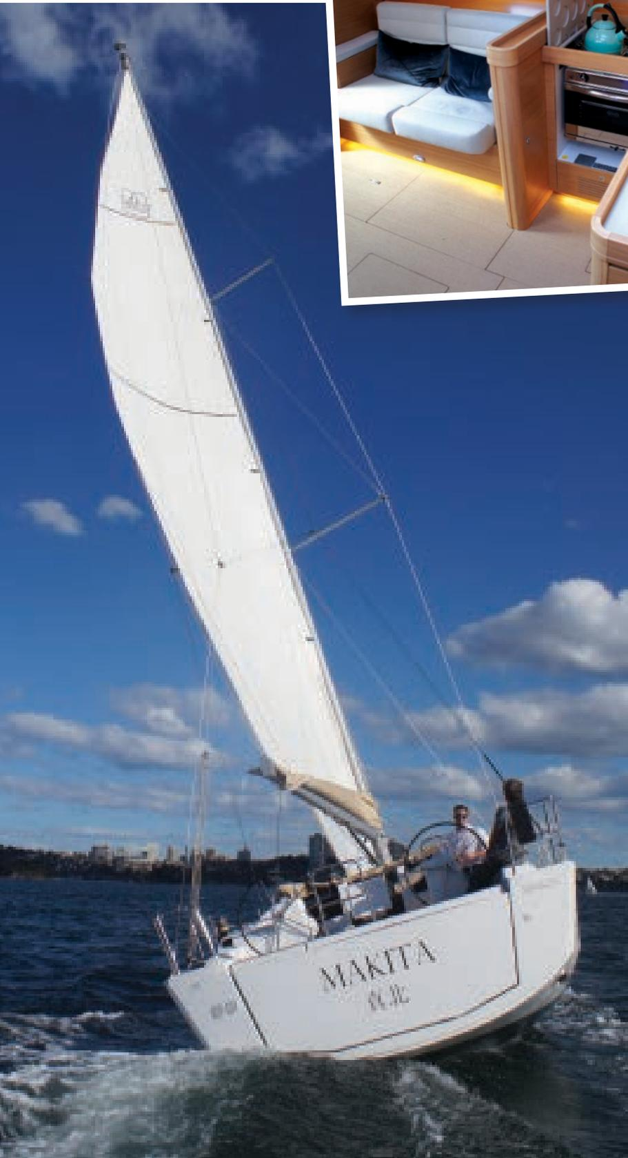
while the sail area is smaller than usual in this class, with its light displacement the sail area to displacement ratio is quite generous.
